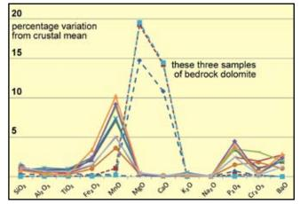
*Figure 5.* Chemical analyses of ten samples of the wad and three of the dolomite bedrock, compared with mean values for upper continental crust.
