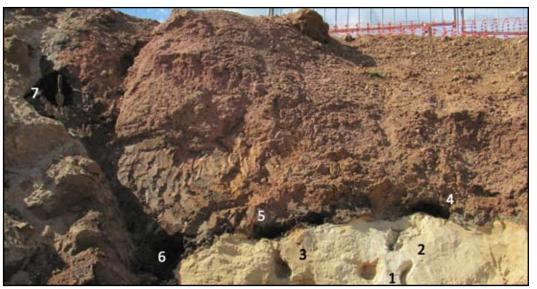
Figure 4. Gradation from bedrock of white dolomite sand, (across the base) to wad above the dark contact, to sediment above the diffuse boundary.
