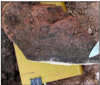
the result of mildly acidic, infiltrating, meteoric water focusing on joints in the bedrock. Sources of acidity for the water include organically derived carbon dioxide and sulphides in the overlying sediment.
